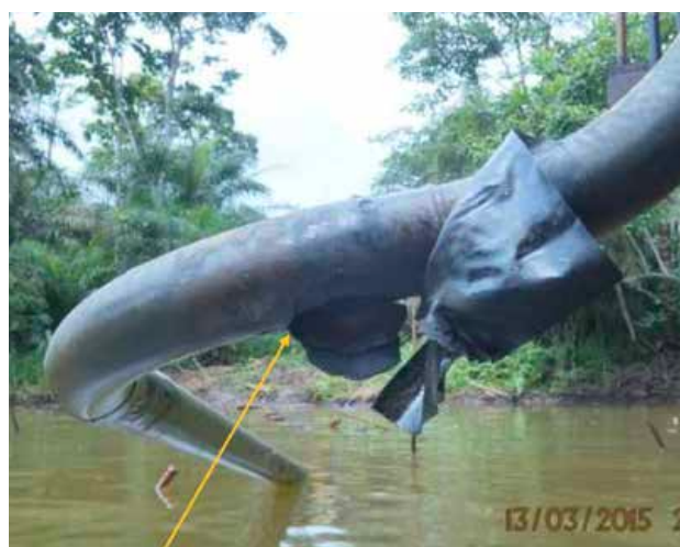
Pipeline tear reported by Shell on 25 January 2015 on its “Seibou Well 2S Flowline at Gban-raun.” Shell reported that the spill was caused by an operational fault, leaking an estimated 549 barrels. Shell photograph.
