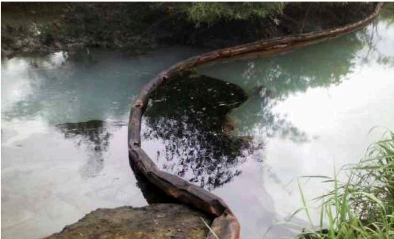
This boom appears to have failed to contain the spread of oil from a spill on the Shell-operated 28” Nkpoiku-Bomu pipeline in 2015. Eni photograph.
