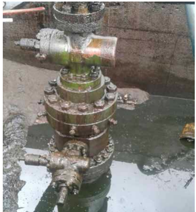
Eni said that "unknown persons" had loosened eight bolts on its well at "Ebegoro 7" causing a spill of 35 barrels on 24 August 2016. Eni photograph.
